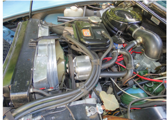
DS 21 carburetor, above . Underhood density fairly typical, but the US air injection pump and pipes add clutter. Unique cylinder head for emissions control may have been incompatible with injection.
