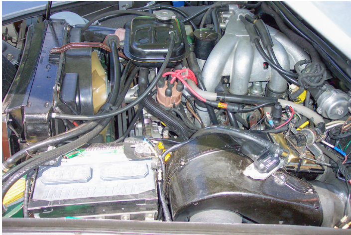
DS Injection engine bay, above . The cast-alloy intake runners just fit beneath the hood profile, but the oil filler neck had to be extended. Jumble of wires at the far left lead to the vacuum sensor and temperature sensors.
