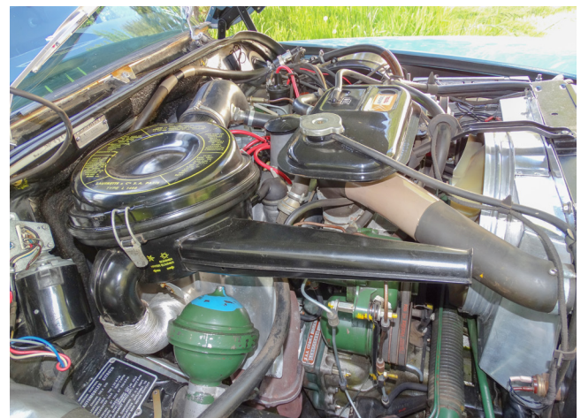
DS 21 carburetor version, above . From this side, completely typical of the type. It is possible to directly adjust the clutch clearance or the centrifugal regulator. Right hand sphere is surprisingly easy.
